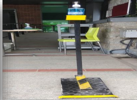
Foot operated pedal hand sanitizer type-3
